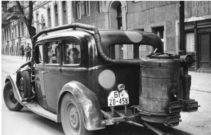
Figure S.8: Car in Berlin 1946. See the “boiler” and the pipe that funnels the extracted wood gas into the internal combustion engine.
